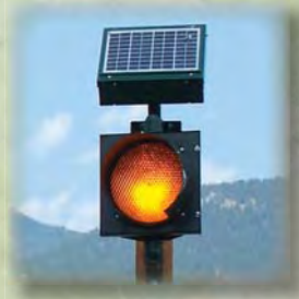
Solar powered beacons on street signs.
