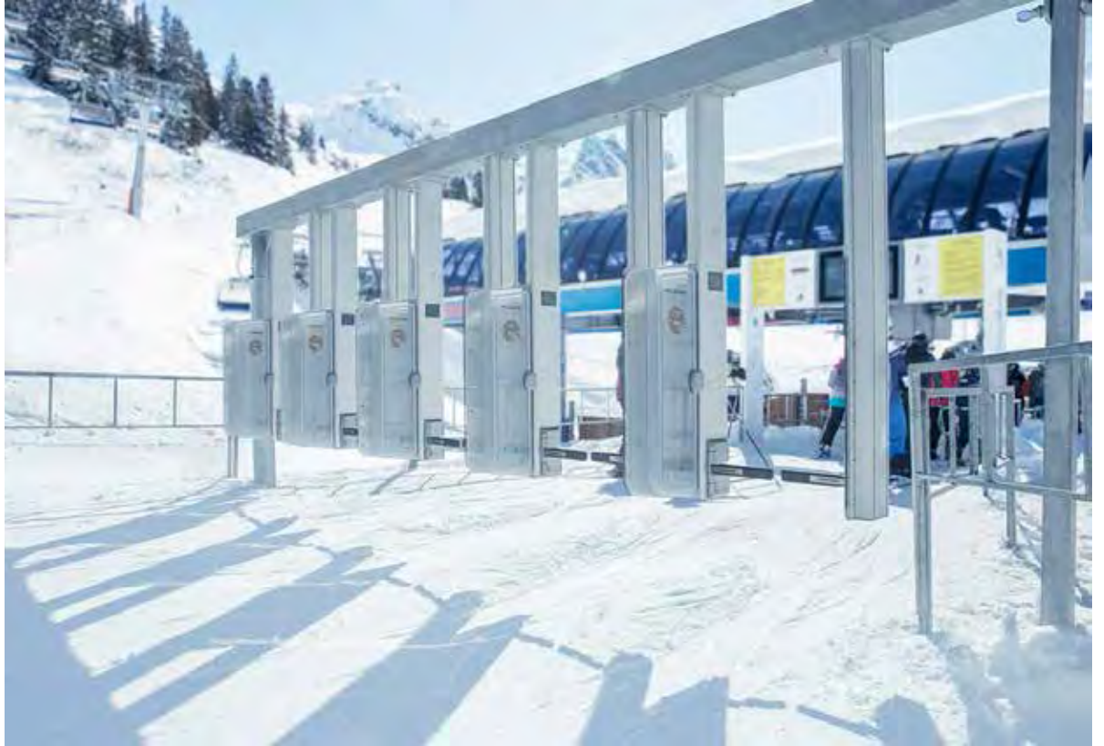
A RFID-equipped gate similar to the ones installed at access points at Big Sky Resort that will allow tickets and season passes to be scanned from inside pockets PHOTOS COURTESY OF BIG SKY RESORT
