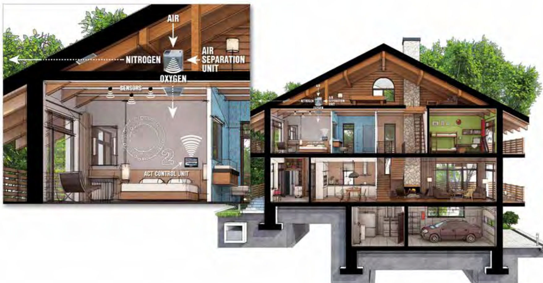
Altitude Control Technology systems consist of air units stored in a mechanical area, a high performance controller for monitoring the space and controlling the equipment, a touchscreen control pad and a small wall port through which the oxygen is delivered. RENDERING COURTESY OF ALTITUDE CONTROL TECHNOLOGY
