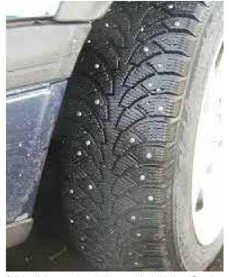
Studded tires like the ones pictured are made with tungsten carbide embedded in the tread. They are best suited to clear ice that's at or near the freezing mark while siped winter tires with softer rubber tend to have better stopping power on snow and in colder temperatures. CC PHOTO
