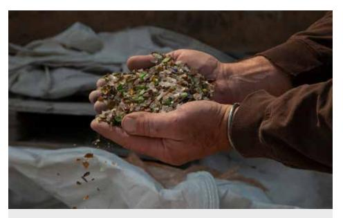
Geomatrix Inc. uses crushed glass shipped from Salt Lake City or Denver and fly ash from a Billings powerplant to make concrete similar to that of the Romans, yet far stronger. PHOTO BY BAY STEPHENS
