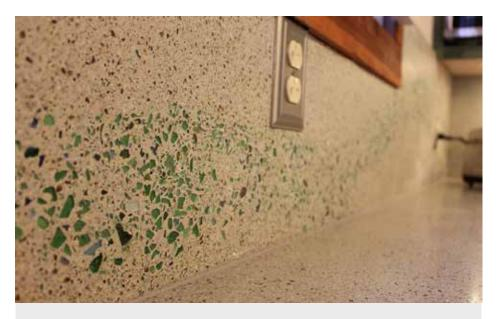
Recycled glass that has been crushed and cleaned flecks the surface of one of Geomatrix's flyash countertops. PHOTO COURTESY OF GEOMATRIX INC.
