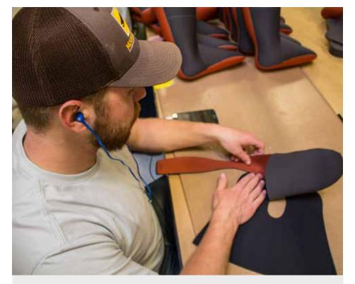
A wader maker glues and assembles pieces of neoprene that will later become the feet of a Simms stocking-foot wader. PHOTO COURTESY OF SIMMS FISHING PRODUCTS
