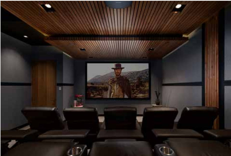
Instead of integrating a 16:9 format screen, SAV used a 2.35:1 screen, which eliminates black bars on the top and bottom allowing for full enjoyment when watching movies in widescreen, cinemascope format. PHOTO BY JON MENEZES
